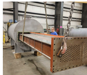
Dual Circuit ES Cooler Bundle Insertion
