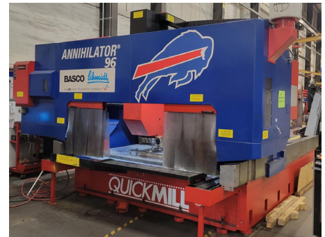
Robotic CNC Machining Center assures precision drilled tubesheets, twenty-four hours a day.
